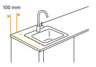
**01** Use a small sink that fits into a 600 mm cabinet. Make sure to have at least 100 mm between the sink and the edges of the worktop to make the construction sturdy.
