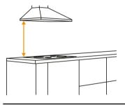
For safety and functionality, follow the recommended height as shown in the assembly instruction for the extractor hood. The height is different whether it is an induction or a gas hob installed in the kitchen.
