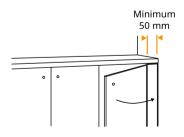
Place a filler piece (minimum 50 mm) between base as well as wall cabinets and the wall to ensure space enough to open doors and drawers fully.
