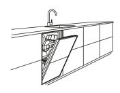
Locate the dishwasher close to the water supply and drain pipes. Having the dishwasher close to the sink makes loading easier and avoids spills on the floor.
